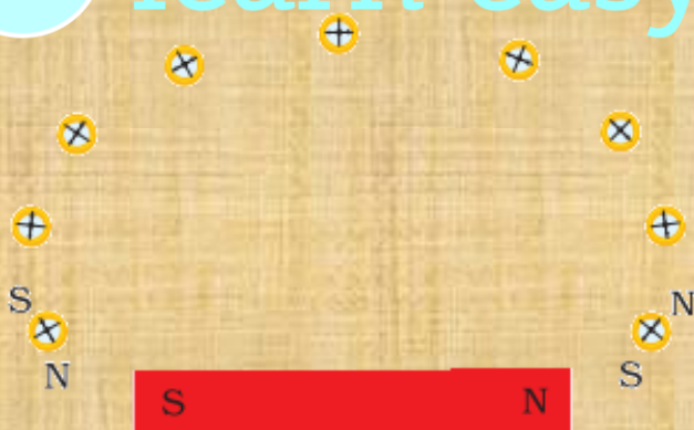
Fig. Drawing a magnetic field line with the help of a compass needle
